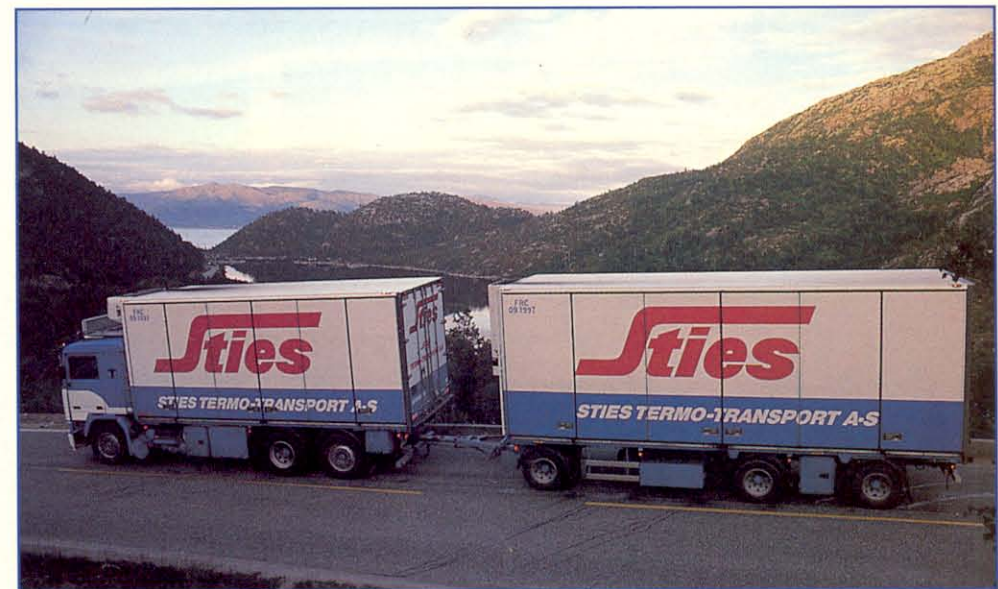
The Sties drawbar is a Norwegian-spec 50-tonner and normally runs at 19.5 metres. It can squeeze down to 18.5 if needed
